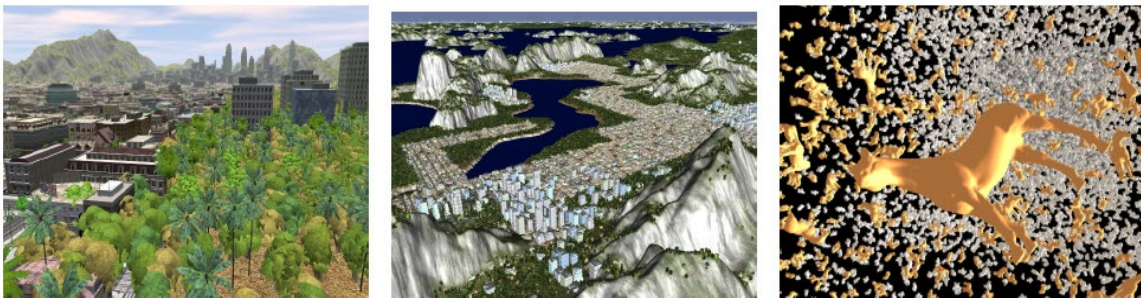
Figure 1: Two scenes rendered interactively over a broadband network on commodity hardware. (Left and center) A 25-billion polygon, 10,000 km 2 Earth-like scene. (Right) A fully three-dimensional scene with 3 billion polygons.
